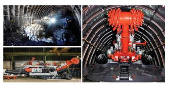
Cutter head in different variations depending on geological condition
