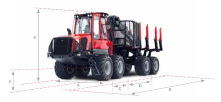
Sturdy balanced portal bogie. Damping bogie
