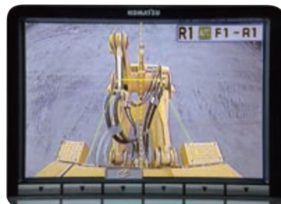
Fully integrated rear-view camera system
