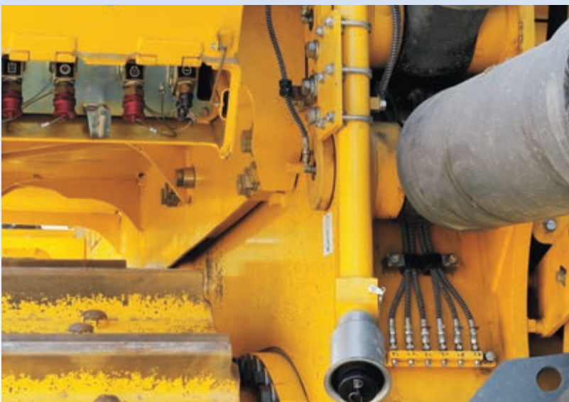
Service center (optional with mining spec) Remote drain ports with couplings and a fast fuel fill connector eliminates the need to get on/off the machine and to remove/install covers to perform fluid maintenance.
