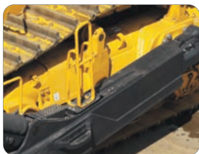
Battery and starter isolator box with jump start receptacle
