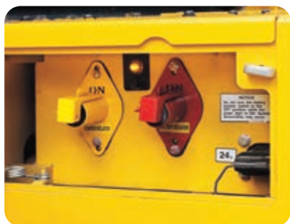
Battery and starter isolator box with jump start receptacle
