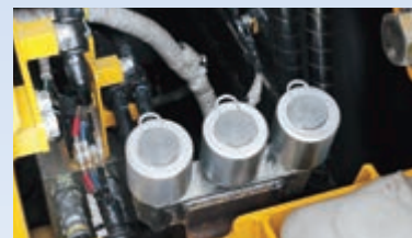
Canister-type breathers facilitate checking and cleaning
