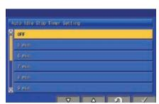
Adjustable idle shutdown automatically turns off the engine after it idles for a set period of time
