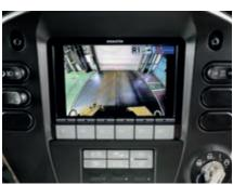
Fully integrated rear-view camera system
