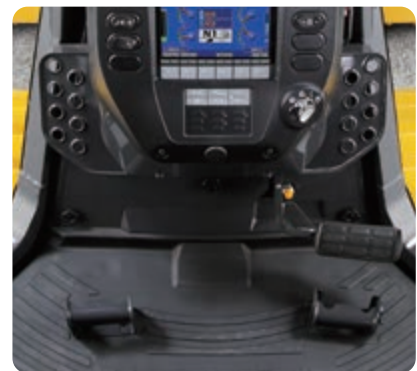
Combined decelerator/brake pedal
