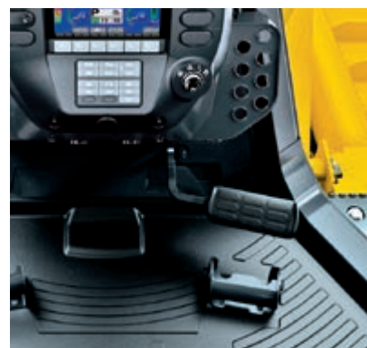
Machine operation is simple with the new one-pedal design that integrates brake function into the decelerator pedal. Machine travel speed can be controlled using one pedal. The pedal function can be changed by a mode selector switch.
