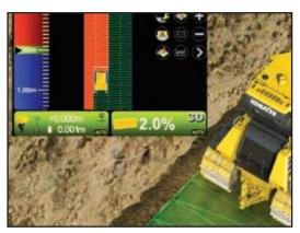
Surface track mapping: cab top GNSS antenna collects accurate "as-built" surface data. It measures actual elevations, as the machine continuously tracks in operation.
