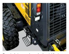
Serrated steps and punched metal foot plate for safe access
