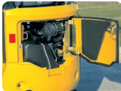
Rear bonnet: quick engine check and fuel tank refilling
