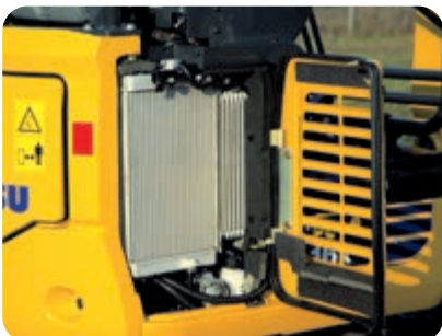
Right bonnet: simple inspection and cleaning of the radiators
