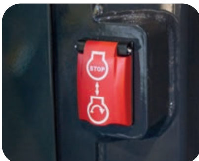
Secondary engine shutdown switch
