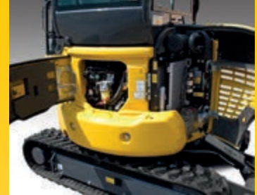
Rear bonnets for quick engine checks, simple inspections, cleaning of the radiators and easy access to the battery
