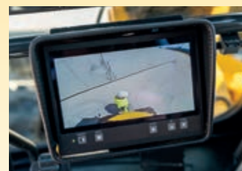
Rear-view camera system (cab version)
