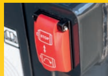
Secondary motor shutdown switch
