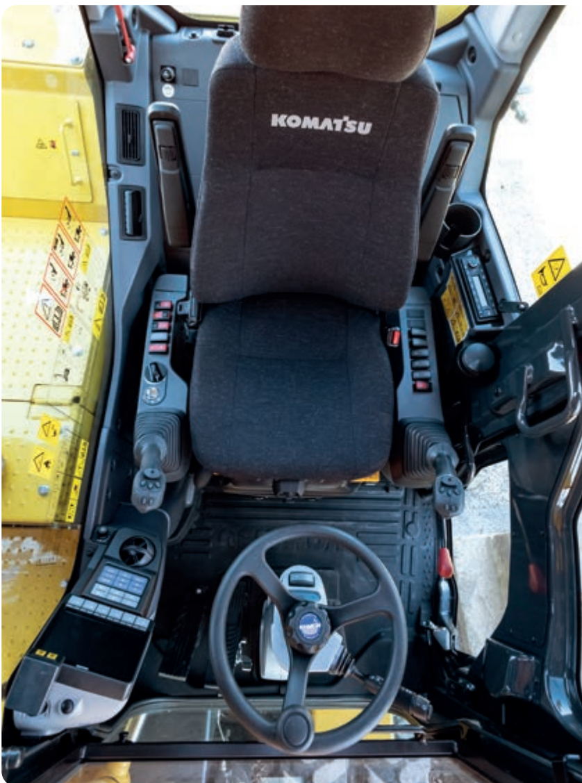
Convenient, ergonomic and precise control: joysticks with proportional control button for attachments
