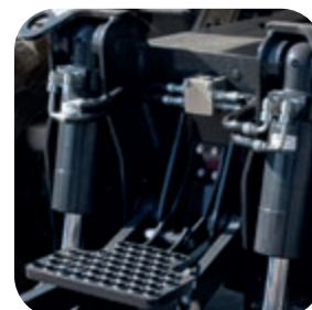
Blade/stabiliser cylinders with integrated check valve (standard)
