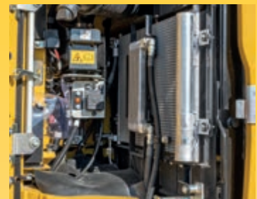
Side-by-side radiator mounting for easy cleaning
