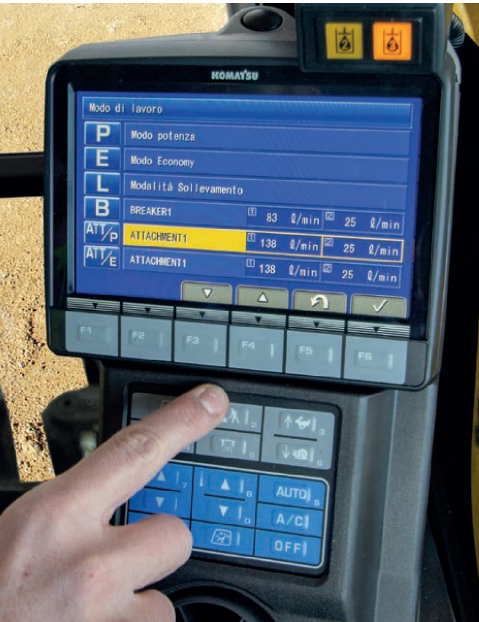
Equipped with universal piping for attachments such as breakers, the conversion to a low-pressure mode requires only a push of the breaker mode switch on the monitor.
