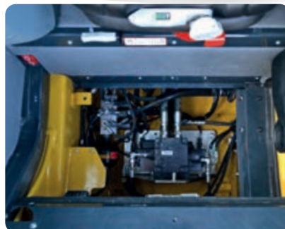
Thanks to the internal cab bonnet, extra servicing of the main valve can be done quickly without tilting the cab
