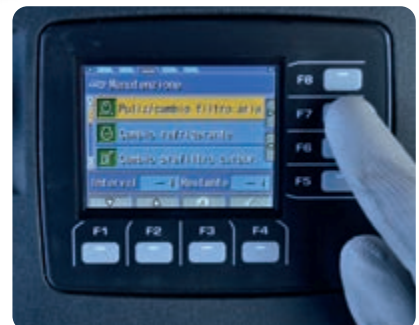
Basic maintenance screen on the 3.5" multi-colour monitor
