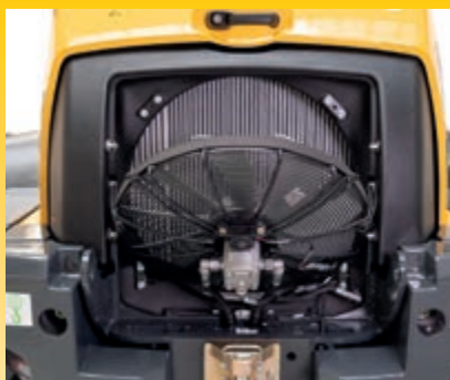
Tiltable radiator fan for convenient cleaning access
