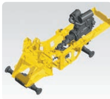
Robust torsion-resistant main frame
