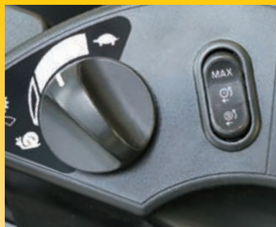
Variable shift control dial with new creeping speed range (left) and variable traction control system switch (right)
