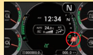
AdBlue® level gauge and refill guidance
