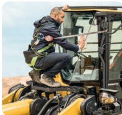
Front cleaning step for safe and easy access to the front window
