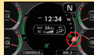
AdBlue® level gauge and refill guidance
