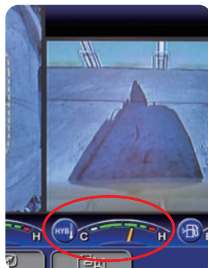
Hybrid system temperature gauge
