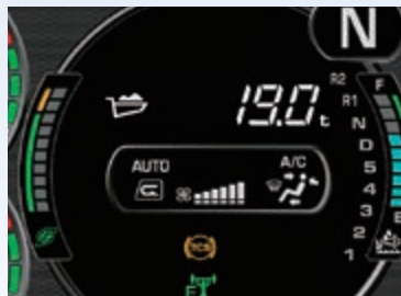
Payload meter displays the loaded weight
