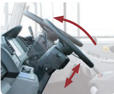
Set the steering wheel to the most comfortable position
