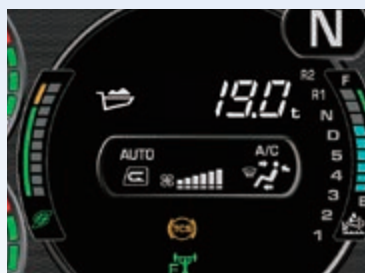
Payload meter displays the loaded weight
