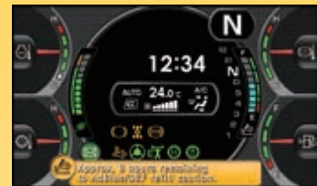
AdBlue® level and refill guidance
