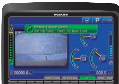
Eco-gauge, Eco guidance and fuel consumption gauge
