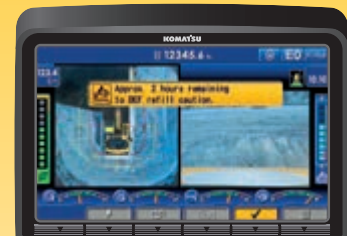
Aftertreatment device regeneration screen for the KDPF
