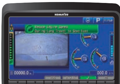
Eco-gauge, Eco guidance and fuel consumption gauge
