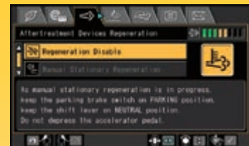
Aftertreatment device regeneration screen for the KDPF
