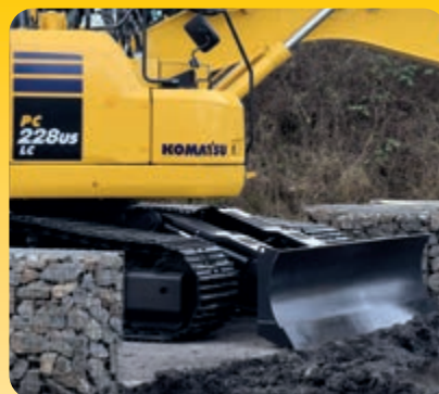
Dozer blade (option) suitable for 600 mm triple grouser (steel) and road-liner (rubber) shoes
