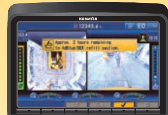
AdBlue® level and refill guidance
