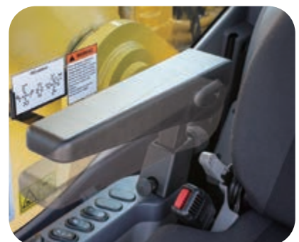
Armrest with simple height adjustment
