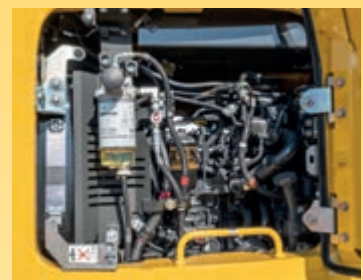
Centralised arrangement of filters
