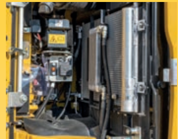
Side-by-side radiator mounting for easy cleaning
