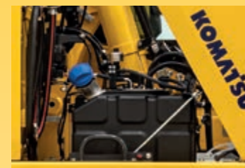
Simple access to the AdBlue® tank
