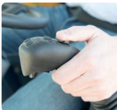
Ergonomic joysticks with proportional controls
