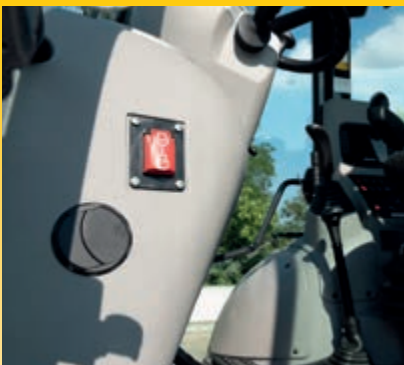
Secondary engine shut down switch
