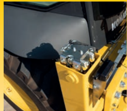
Anti-burst valves for stabilizers, boom and arm (Standard)
