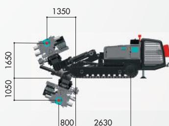
\* Rig movements are the maximum allowable. Any additional equipment on the rig may limit these movements.
