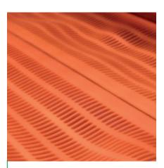
Aggressive flip-flow bottom deck. Variety of mat sizes available. Secured with friction wedges, no securing bolts.
