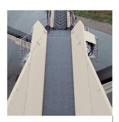
Heavy duty, abrasion resistant, steel apron feeder as standard.
