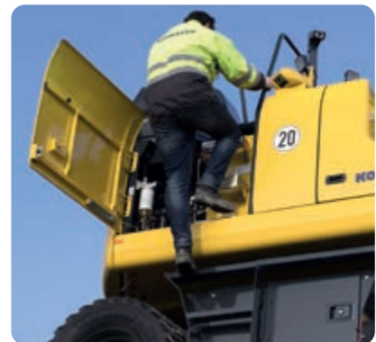
Handrails and anti-slip plates
