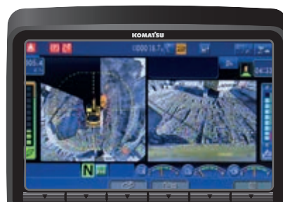
With KomVision, various camera view options help to maintain a constant bird's eye view from above the machine
