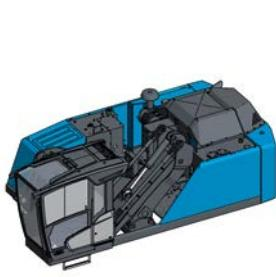
Cab system vertically adjustable and horizontally adjustable
