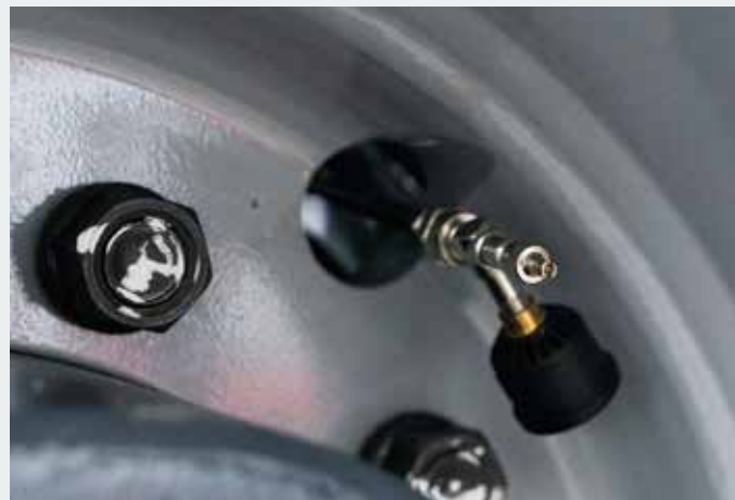
• Wireless tyre pressure monitoring
