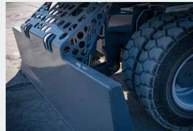
• Support blade, integrated cylinder protection
