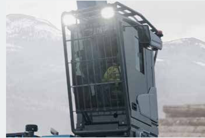
• Front and roof guard for timber application
