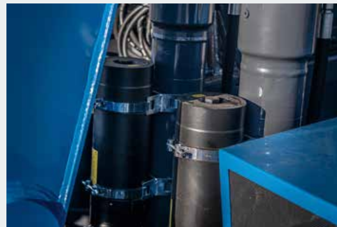
• Boom cylinder damping system
