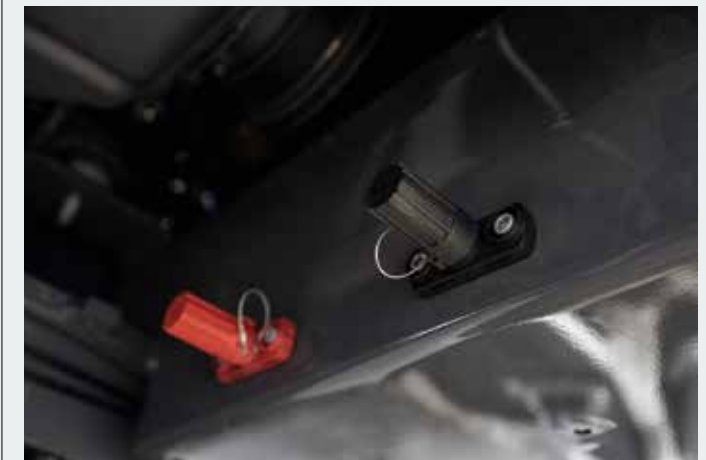
• External battery terminals
