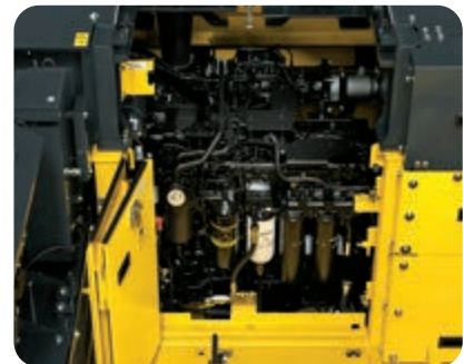
Centralised arrangement of filters
