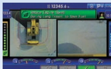
Eco-gauge, Eco guidance and fuel consumption gauge
