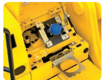
The AdBlue® tank is installed on the front stairway. The included workbench makes refilling AdBlue® even easier.
