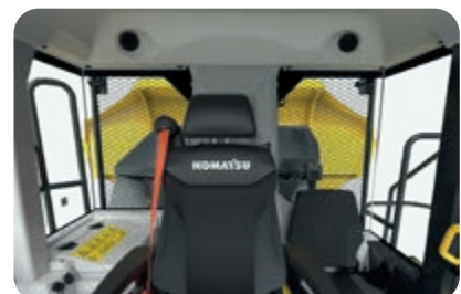
Rear visibility has been enhanced by removing the rear-left and rear-right pillars
